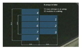
Fig. 1. FPV arrays layout
